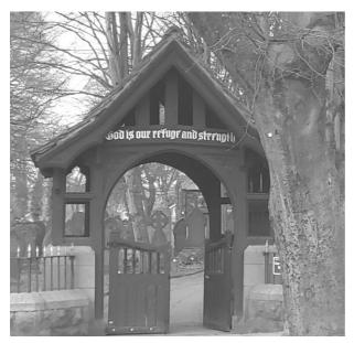
For the last couple of months, the churchyard team have been working on the lychgate at Christ Church. We have refurbished it beginning with sugarsoaping, to remove the dirt and grime which have accumulated over the last century, then reoiling the oak frame. We retrieved the gates
